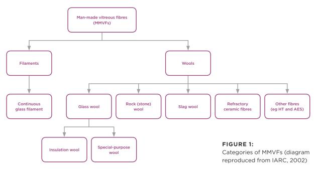
HT = high-alumina, low-silica wools; AES = alkaline earth silicate wools
