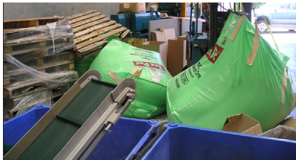
Picture 3: this photo shows one super sack in the background stacked alongside the concrete wall (partially obscured by pallets and second super sack). Super sack 2 has fallen over, to land in front of super sack 1. Super sack 3 is the sack that crushed the worker. The bag's straps are hanging on the forklift's tines (the forklift was used to move the bag off the worker).
