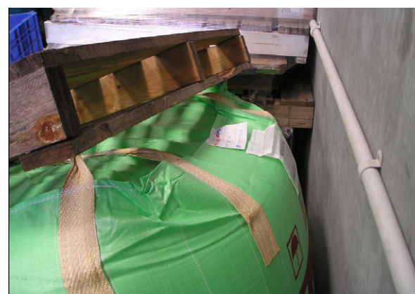
Picture 2: this photo displays the compression to a lower-stacked super sack from the bag that was previously stacked on top.
