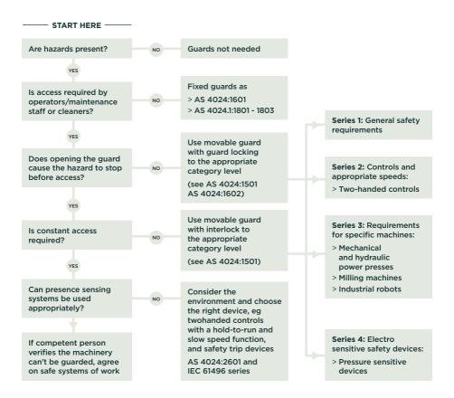
Note: the flowchart does not take other protective devices, such as two-hand controls, into account.
